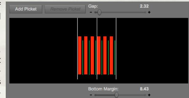
We also adjusted the bottom margin to 8.43 DS units (cm), to give the fence a little air between the fence and the ground below. It's good to keep in mind that the Posts all have a 20 DS units extra below ground, to handle cases of uneven ground. The display here shows from ground and up though.
